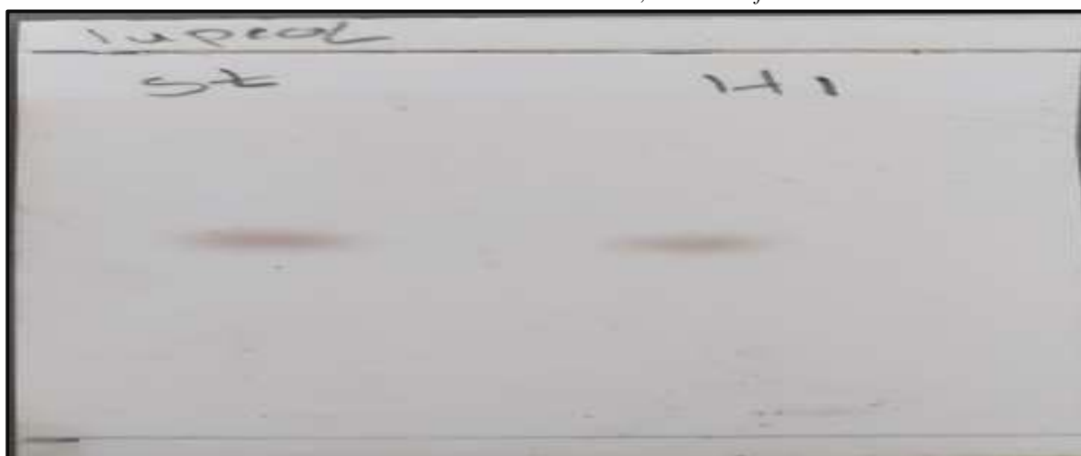
Figure 7. Thin layer chromatogram for isolated compound (H1), with lupeol std. Standard and the Corresponding Detected Compound H1.
